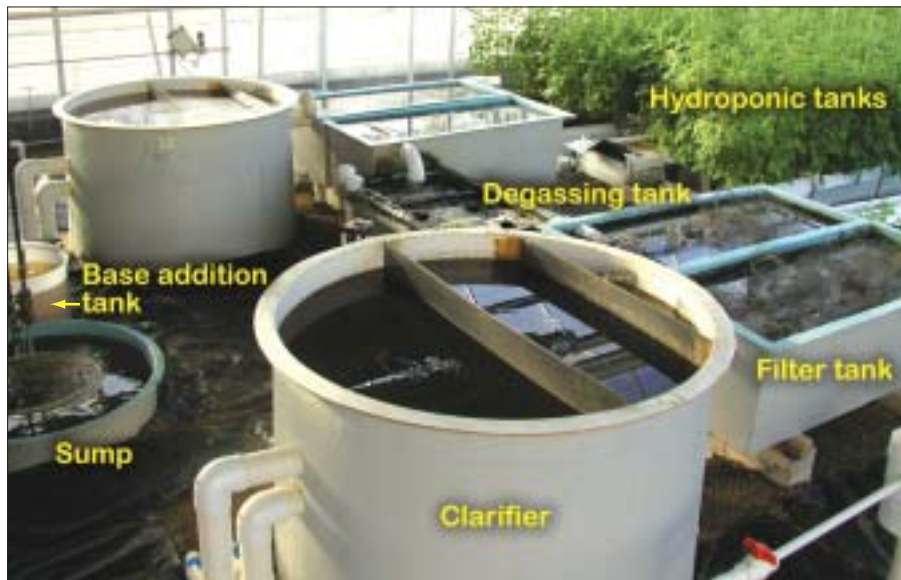
Figure 7. Components of the UVI aquaponic system at the New Jersey EcoComplex at Rutgers University.
